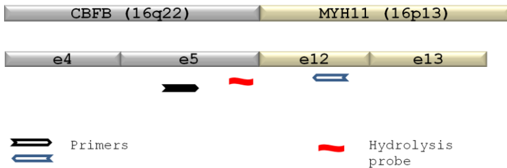
Figure 1: Annealing locations of the PCR primers and hydrolysis probe
